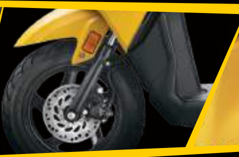
Telescopic Suspension & Front Disc Brake
